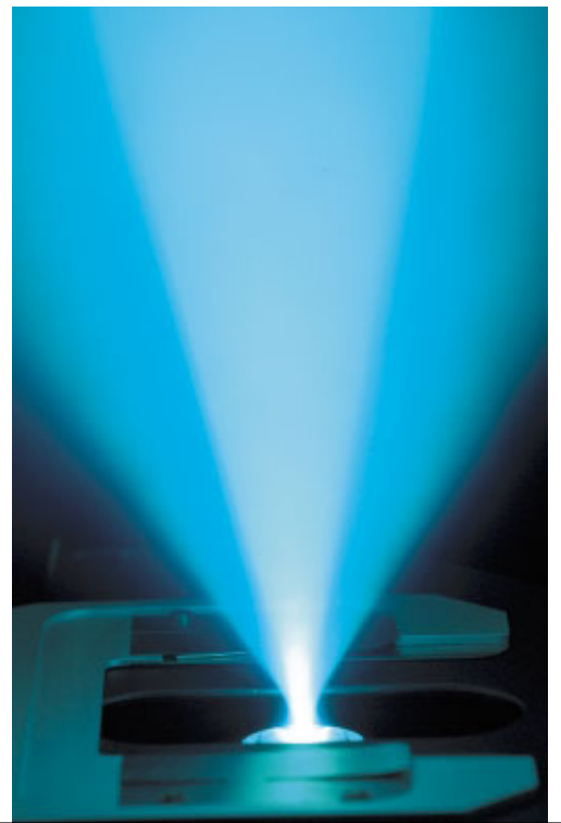
Condenser aperture automatically matched to the objective aperture
