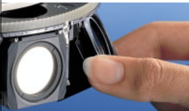
Change of filter cubes – the Push&Click technique
