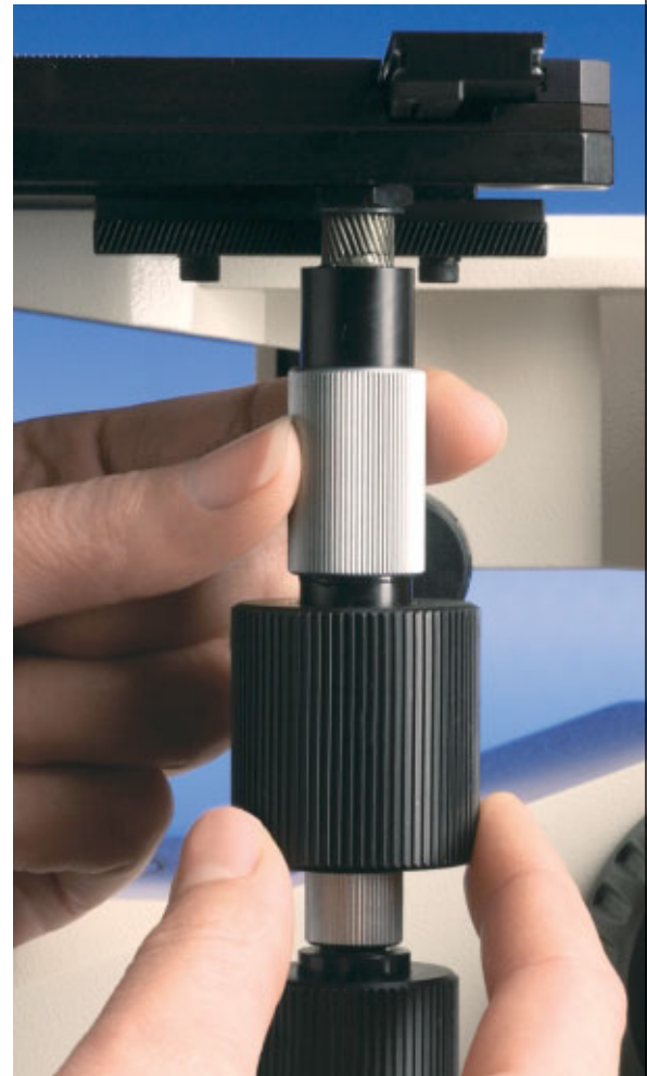
Vertically adjustable control elements on the stage drive
