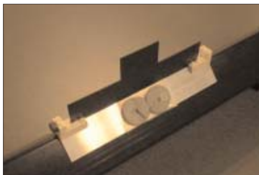
Figure 9. Linear air track vehicle for collision experiments.
