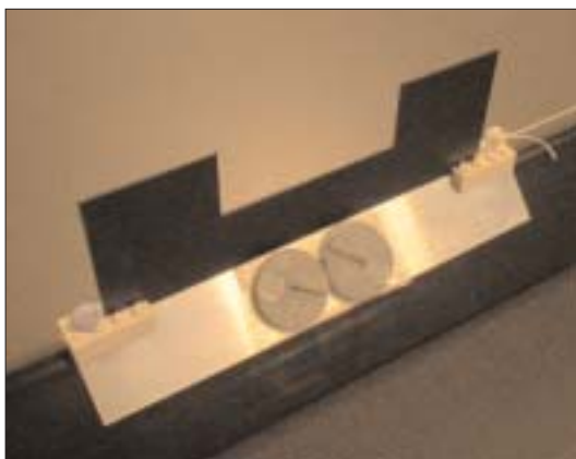
Figure 10. Linear air track vehicle for force, mass and acceleration experiments.
