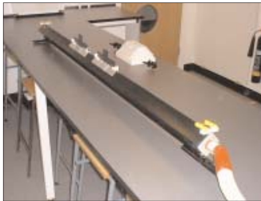
Figure 1. Linear air track set up for collision experiments.
