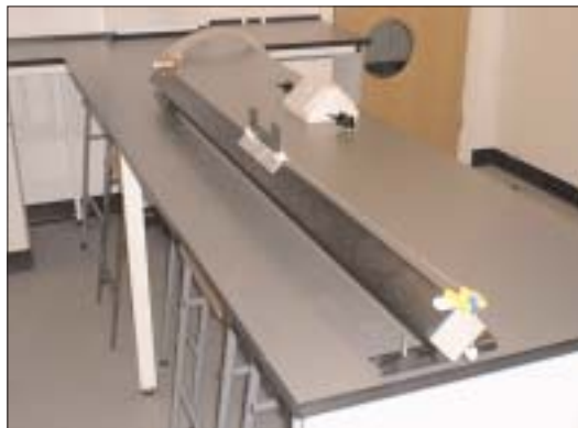
Figure 2. Linear air track set up for force, mass and acceleration experiments.
