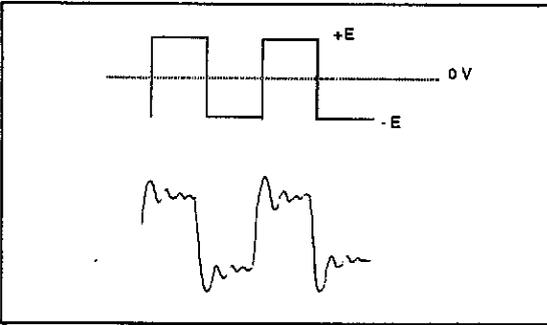
Figure 2. Typical input (top) and output (bottom) waveforms observed in the circuit shown in figure 1.
