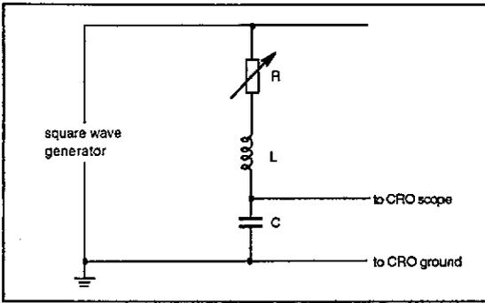
Figure 1. A simple circuit for showing the oscillation of electric charges.
