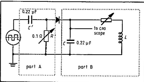
Figure 3. A modified circuit connection for showing oscillation of electric charges.
