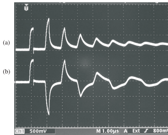
Figure 6. Multiple reflections in the ‘coaxial cavity’ configuration corresponding to (a) open end and (b) short circuited end.
