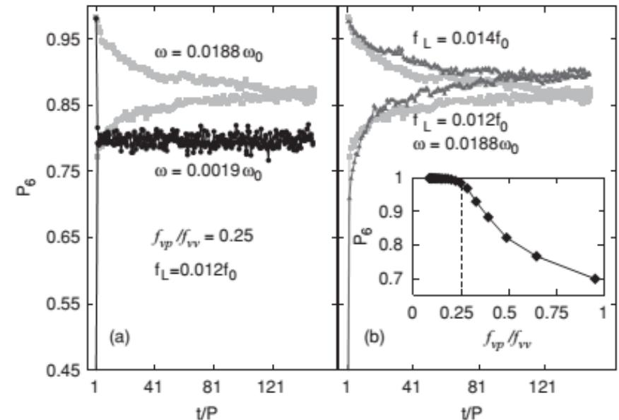
FIG. 4.  $P_6$  versus  $t/P$  starting from an ordered and a disordered configuration. (a) For two different  $\omega$  and fixed  $f_L$ . (b) For two different  $f_L$  and fixed  $\omega$ . (Inset)  $P_6$  versus  $f_{vp}/f_{vv}$ , showing a spontaneous creation of disclinations, and a decrease in  $P_6$  at around  $f_{vp}/f_{vv} = 0.25$ .
